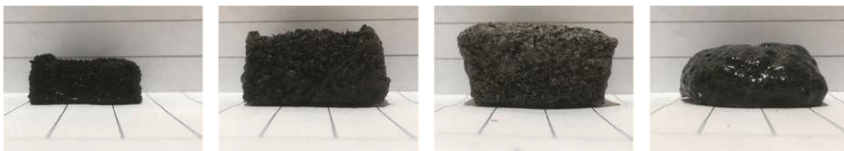
Fig. 7. Results of the silicate material heat treatment at various temperatures (from left to right): Original silicate; 250 °C; 550 °C; 920 °C.
