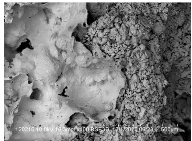
Fig. 14. Cross-section of the cellular ceramic material, scanning electron microscopy.
